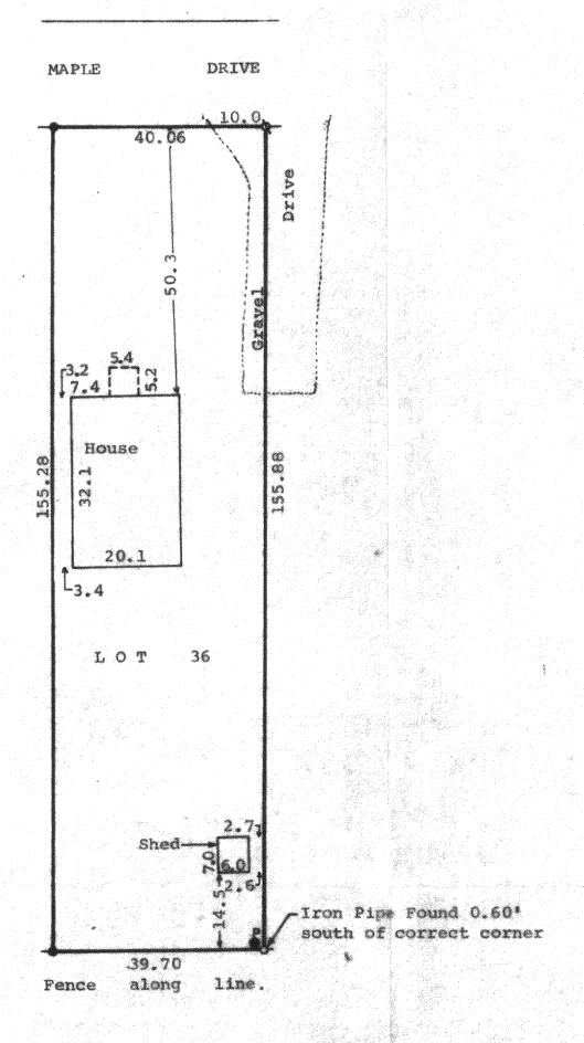
Scale - 1" = 20q = Iron Pipe Found Bent and Reset O = Iron Pipe Found e = Iron Rod Found
